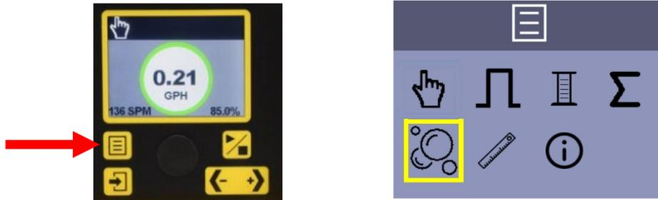
2. Press the right arrow button (6) to put the yellow box over the "External Pulse Mode"
