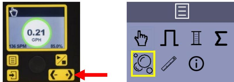
3. Press Enter (4) to access the "Stay Prime, Degassing" operation
