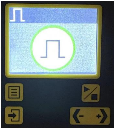
Pump is on and awaiting signals from the flow meter and FS-1 Switch Box.
