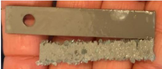
Clearer view of the sulfuric acid coupon
