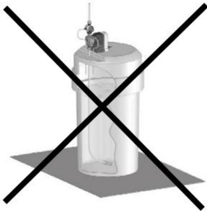
INCORRECT Foot Valve tilted sideways WILL NOT PRIME
